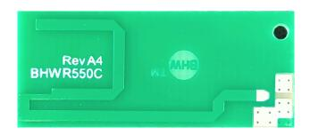
12x30x0.6mm PCB for IPX/UFL Cable Assembly
